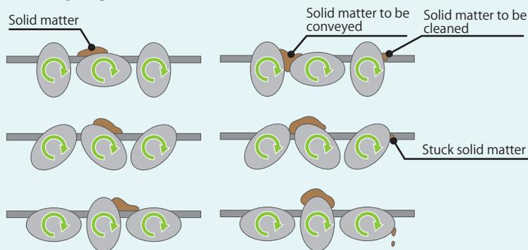
Oval plates push down the stuck solid matter to keep the filtering zone clean.
