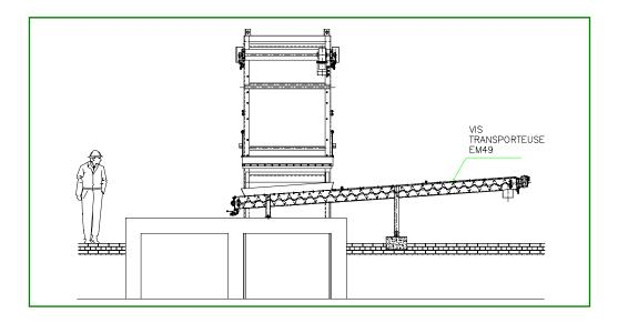
• Screw conveyor EM49, with or without central shaft, UHMW-PE wear surface, directly connected worm gearbox, carbon steel or stainless steel made.
